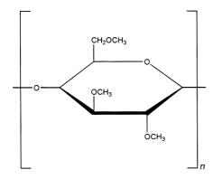
The structure shown is with complete substitution of the available hydroxyl units of methoxyl substitution. Note that methoxyl substitution can occur at any combination of the hydroxyl groups of the anhydroglucose ring of cellulose at positions 2, 3, and 6. *See* Section 4.
